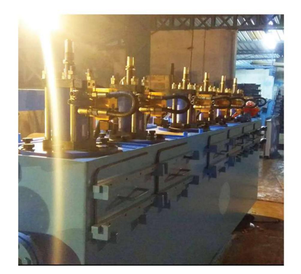
Pneumatically operated cylinders with discharge gates controlled by the density sensors and total system managed by the PLC settings ensure that the Stratification of the different density material takes place quickly and finely resulting in precise cutting of the product in the process operations. Benefits to the customer are higher yields and minimum misplacement.
