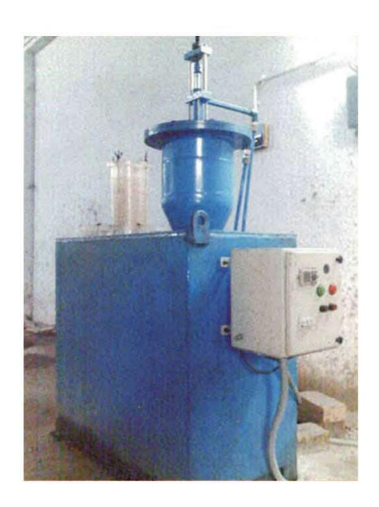
Test unit available for conducting the bench scale tests to determine the amenability for gravity separation, sizing parameters and PLC settings.
