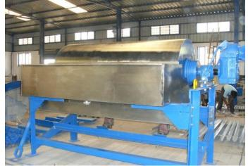
The designs offered include Multipole and Interpol magnetic arrangement systems and carefully selected to suit the customers' process requirement.
