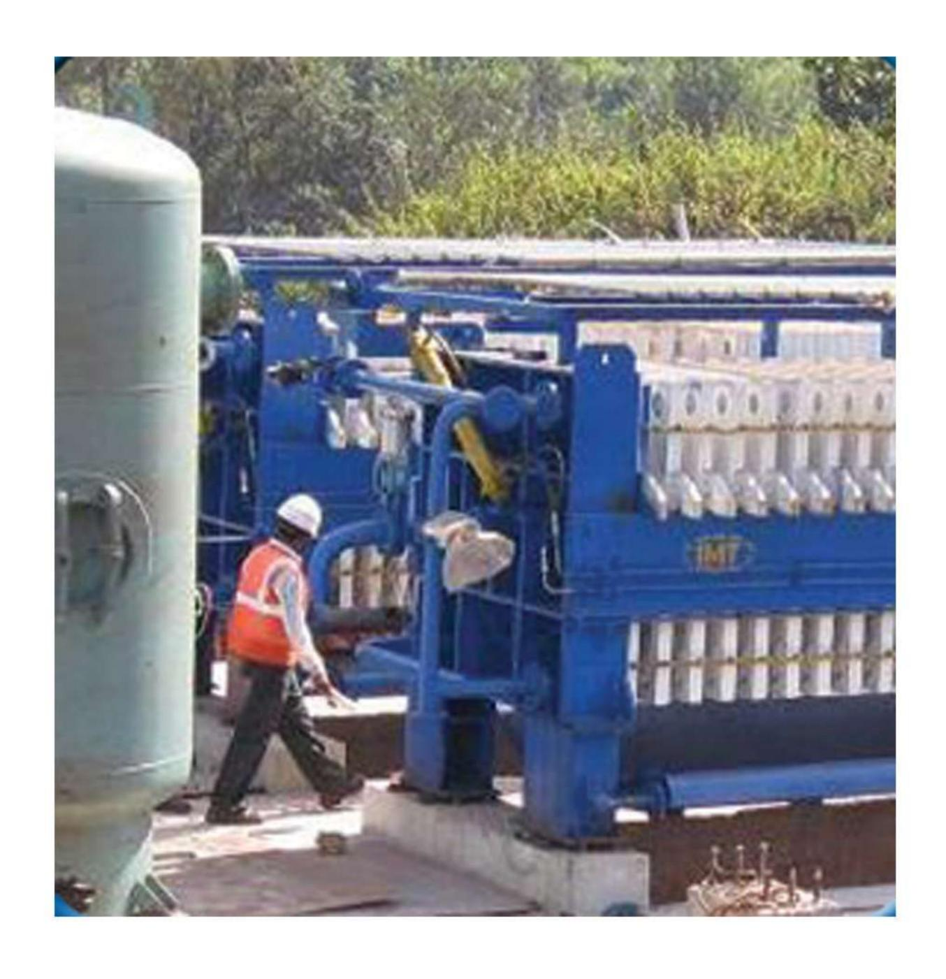
Tailings disposal is always an issue in mineral processing industries and **IMT** is providing solution to this by developing indigenously designed and manufactured fully automatic pressure filters to the customers. The PLC controlled operations of the pressure filters provide the option of using the same for concentrate filtration also, if need be.
