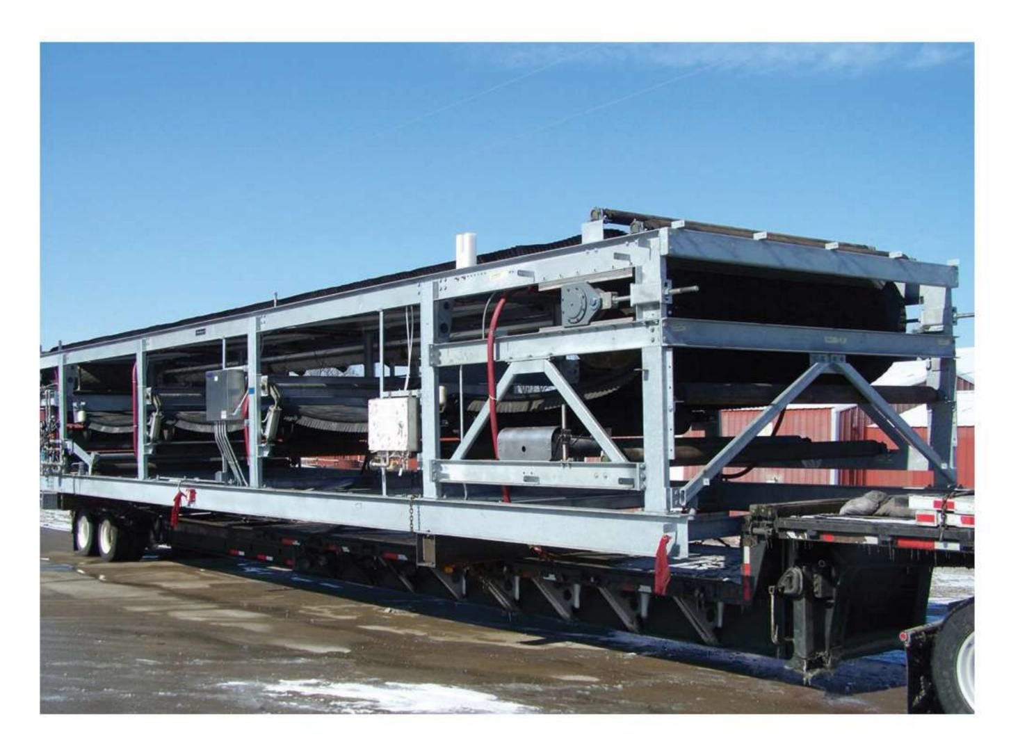
Horizontal belt filters are extensively used for filtration of Concentrates and Tailings in Iron ore, Coal, Phosphoric acid filtration, Di Calcium Phosphate filtration and many other mineral and chemical applications.
