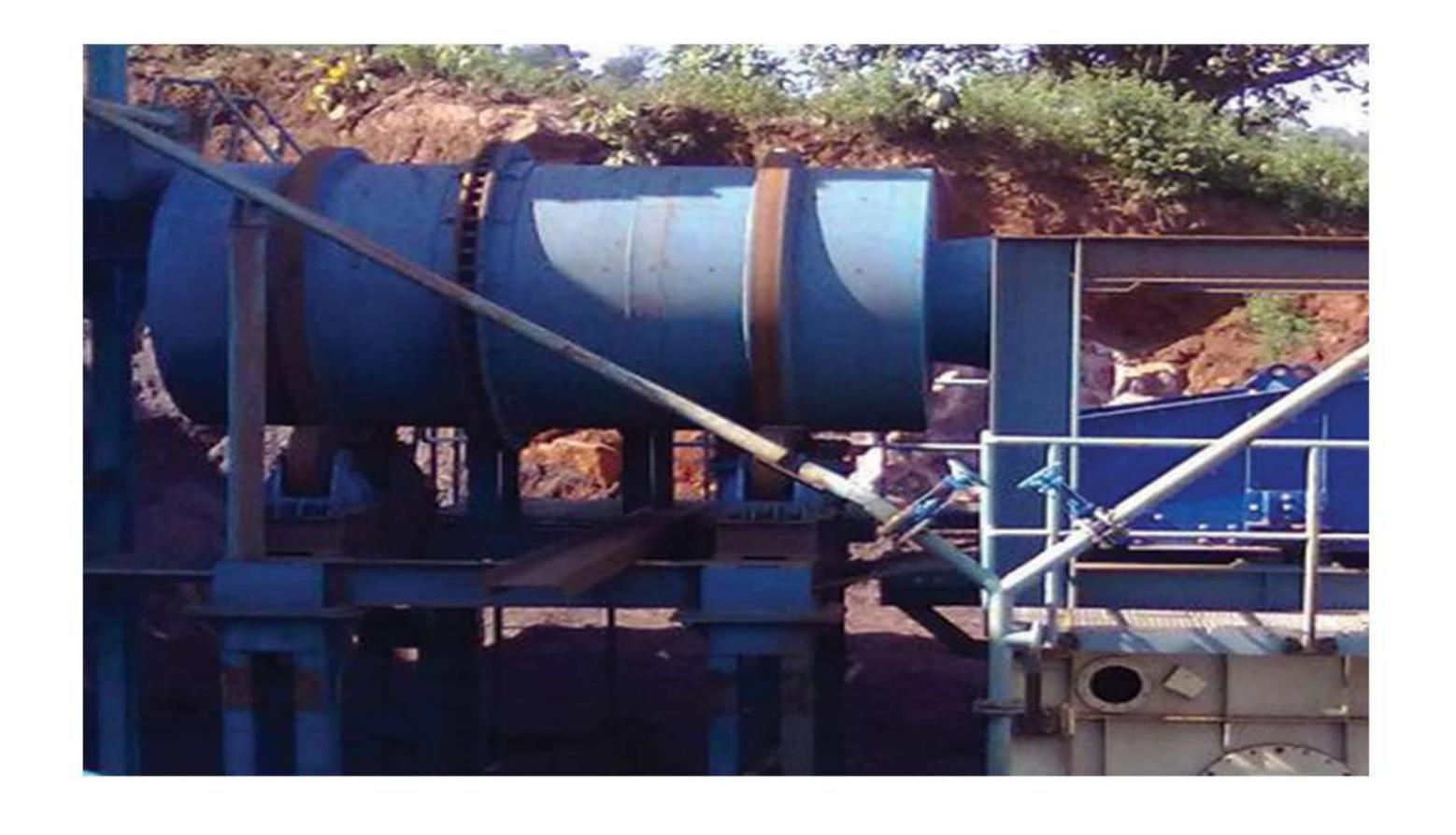
IMT offers drum scrubbers to complement its other products and has successfully installed and commissioned drum scrubbers for iron ore applications up to 250 tph capacity.
