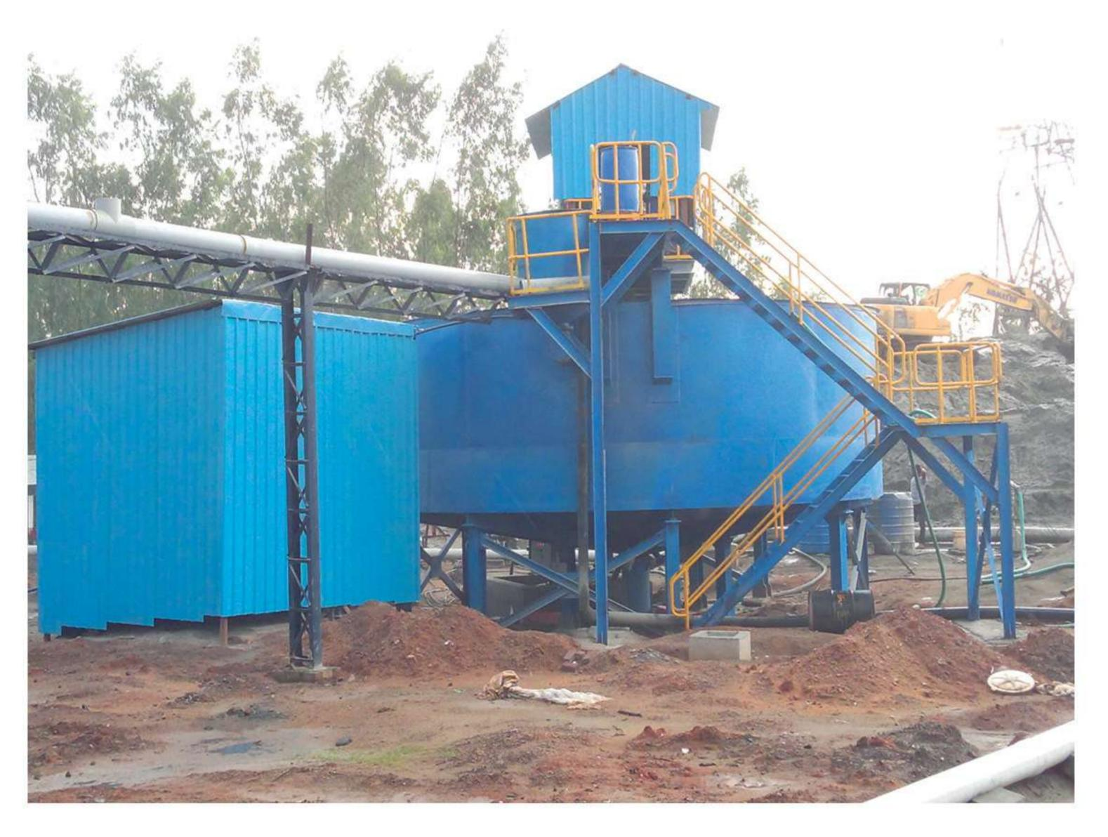
High rate thickeners are one of the important equipment for efficient recovery and recycling of water in Mineral processing plants and IMT has specialised in offering IMT thickeners with sizes starting from 3 m to 60 m. Designs are available for manufacturing up to 100 m diameter. Thickeners with Steel construction tanks are available with each and every design going though Finite element analysis to ensure that the designs are robust and economical.
