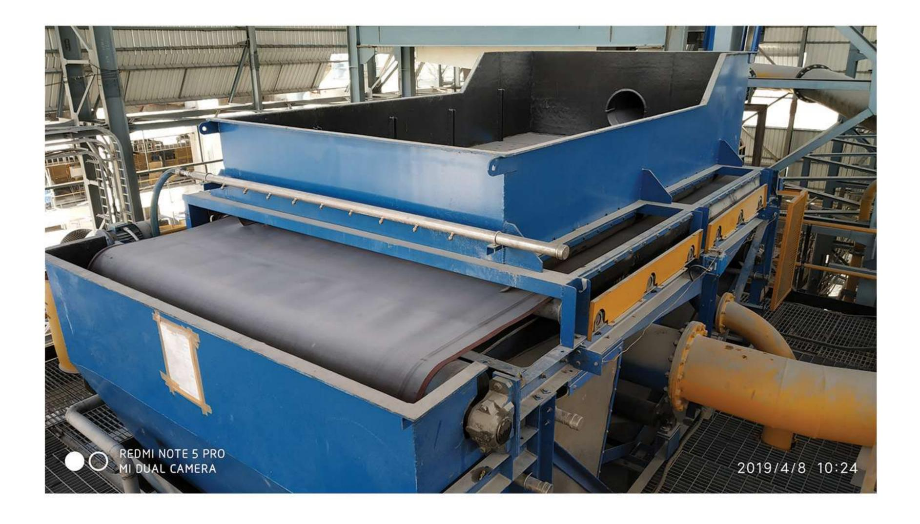
Linear Trash Screens are extensively used in the mineral processing industries as a protective equipment prior to Thickeners and High Intensity Magnetic Separators in the Gold leaching plants, Iron Ore processing plants etc.
