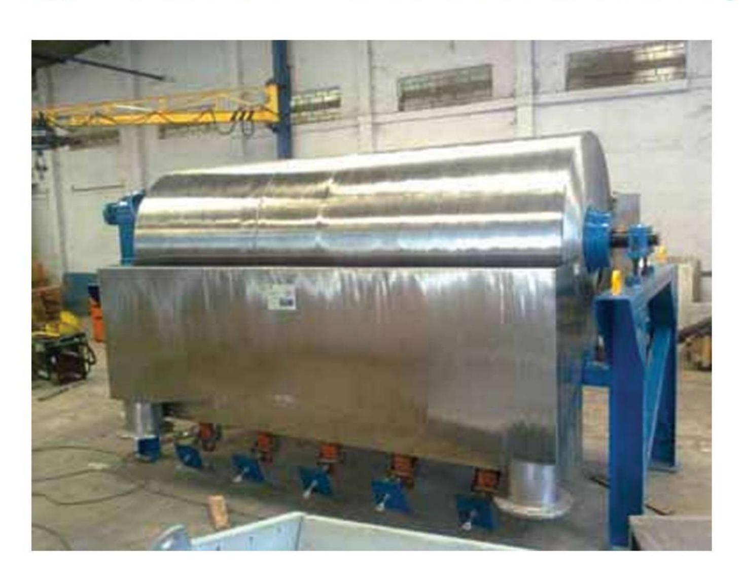
Low intensity and Medium intensity magnetic separators are offered by IMT with the technology support from Malvern engineering company, South Africa on case to case basis. The range offered for Low Intensity Magnetic Separator is up to 2500 gauss and for Medium intensity Magnetic separators it I up to 6000 Gauss. The drum diameters starting from 305 mm to 1220 mm and the length of the drums up to 3050 mm.
