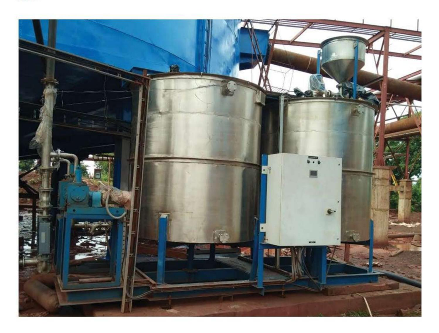
IMT offers Fully Automatic Flocculent and Reagent Dosing Systems as stand alone product as well as part of the High rate thickeners and Flotation cells. Sizes offered vary from 1.0 kg/hr to 50 kg/hr dosing of the Flocculants/ reagents.
