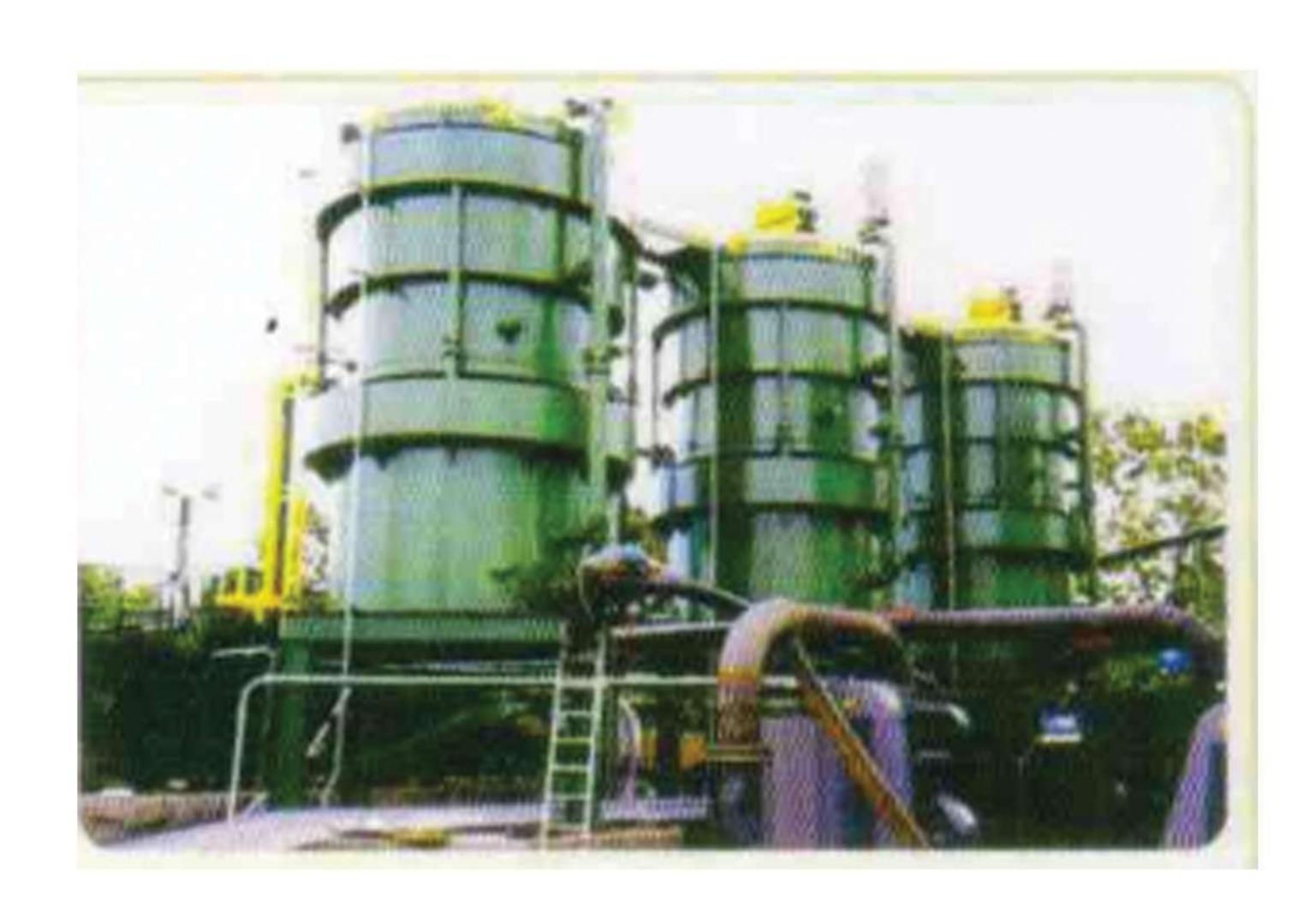
Maxflot Ltd has acquired Beneficiation technologies Ltd, USA which has patented designs for Duel extraction column flotation cell for froth flotation applications. DEC has unique features such stub column flotations mounted one top of the other and thus scavenging/ cleaning application is carried oout in a single unit. Successful installations are in Coal flotation, Silica flotation and Iron ore reverse flotation applications in the world.
