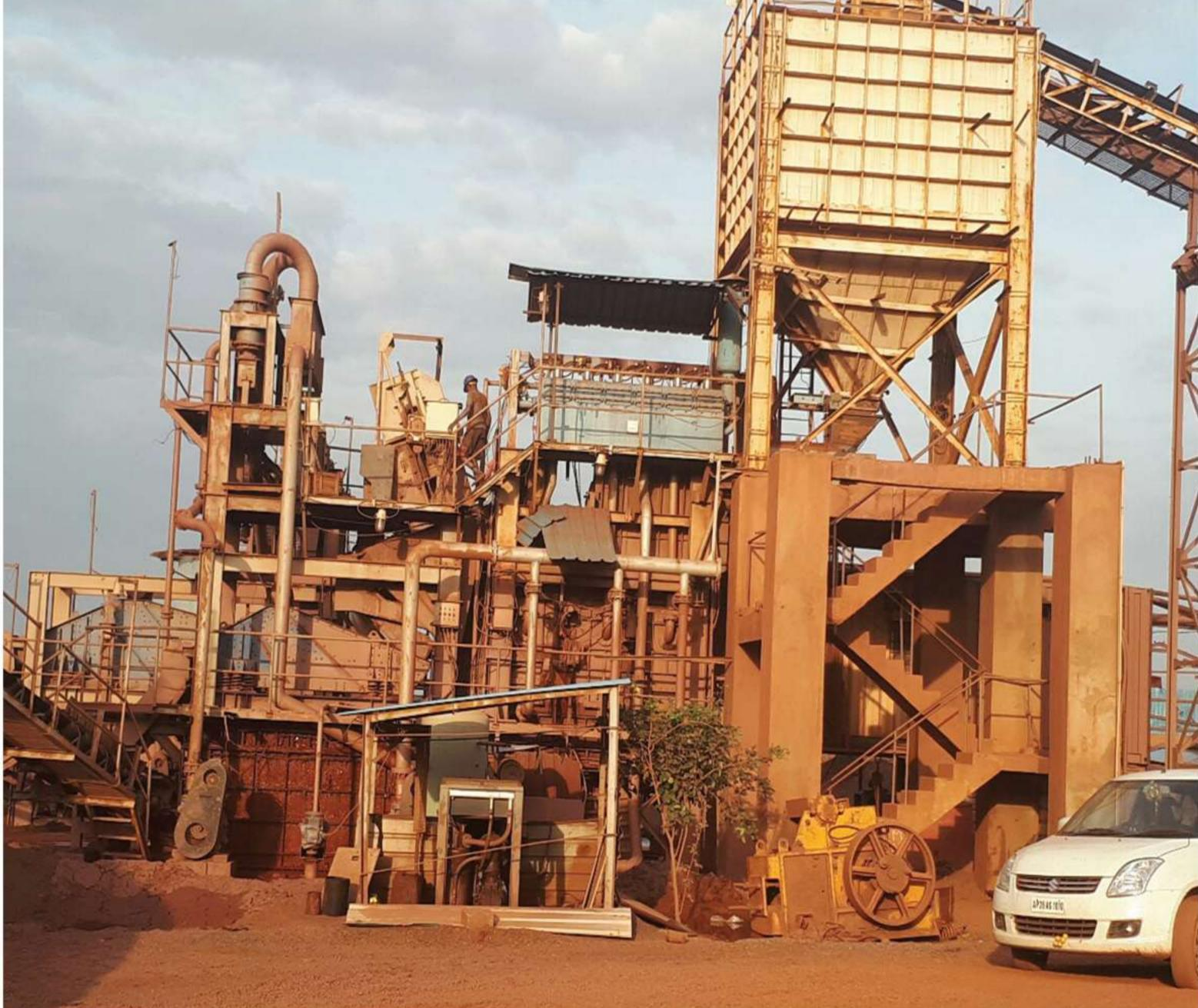
IMT is the first company in India to offer a modular Baby Jig plant with complete system from receiving hopper to the discharge conveyors mounted on fabricated structures. A typical Baby jig plant can be supplied, erected and commissioned within a period 3-4 months depending upon the customers ability to complete the civil foundation works.
