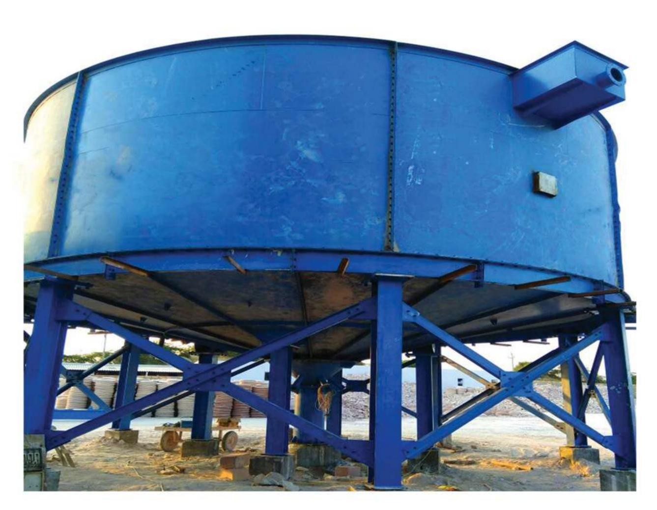
**IMT** has developed bolted construction design for the thickener tank and tank supports up to **14 m** diameter which reduces the construction time and for fast gestation projects this design is well suited. Other advantage of bolted design construction tanks are the thickeners can be relocated easily when the project operations require shifting from one point to another.
