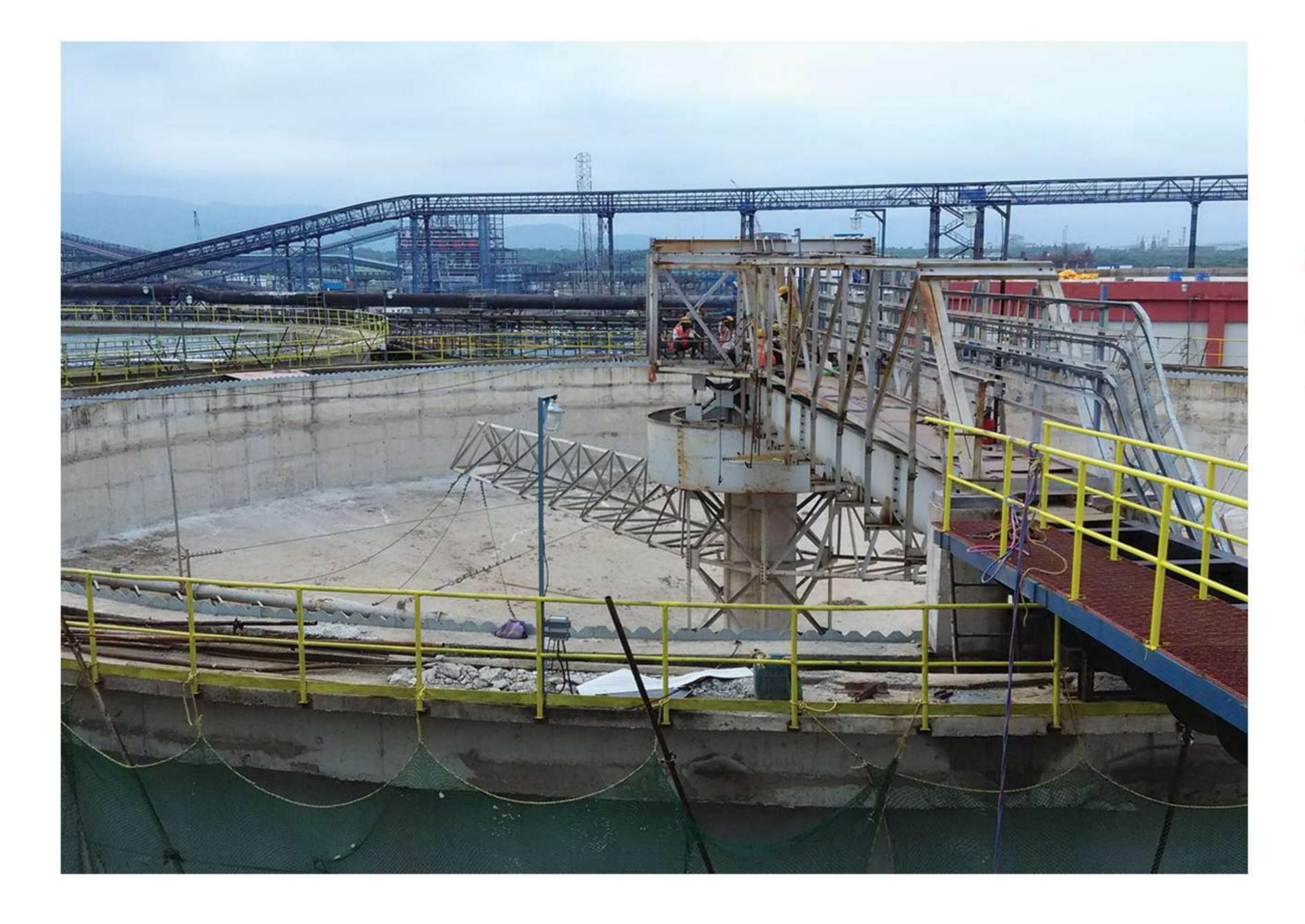
IMT has developed cable torque thickeners for lighter duty applications where the underflow solids concentration does not exceed 20- 25% and typical applications are chemical industry effluents, Blast furnace dust and even for Coal tailings.
